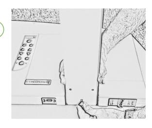
Mount Camera arm into guide holes and fix the 3 black screws
