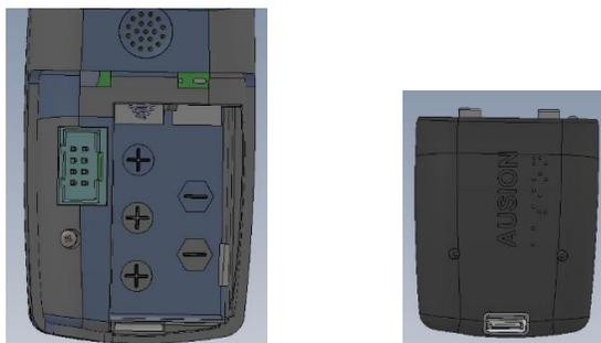
Figure 2. Battery Compartment and Cover
